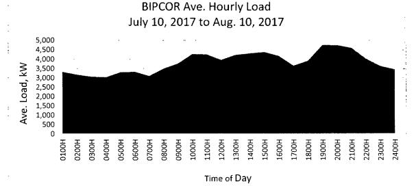
Note: Minimum load demand was 2,950 kW @ 0700H on 10 July 2017 Maximum load demand was 5,350 kW @ 1930H on 09 August 2017
