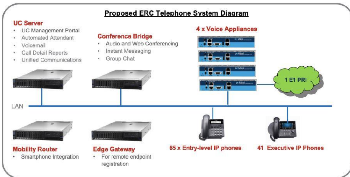
Figure 2. Proposed ERC Telephone System Upgrade Diagram
